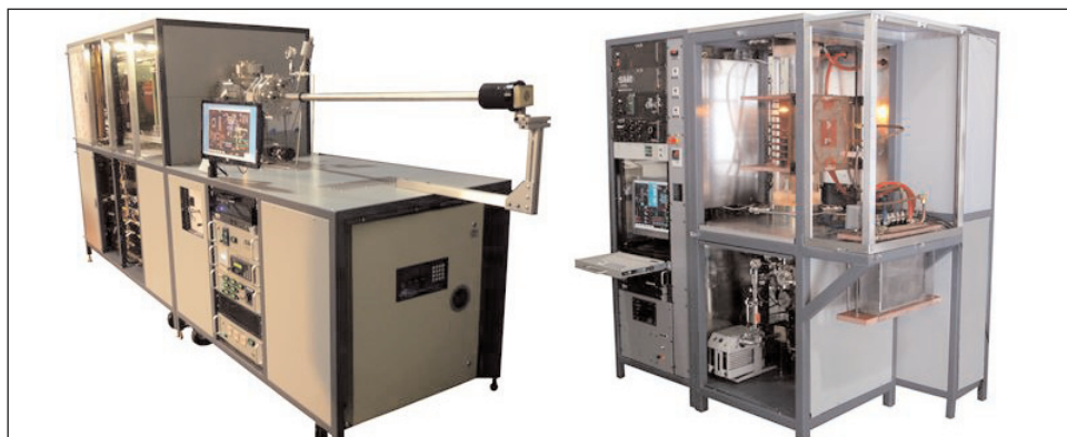
Previous SiC horizontal (left) and vertical (right) reactor systems built by SMI for the US Naval Research Laboratory and Penn State University, respectively.
