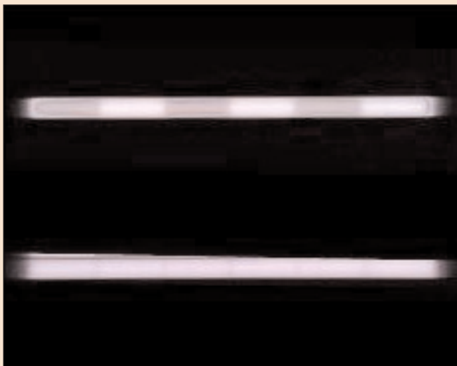
Top: inconsistent LED performance when dimming. Bottom: Smooth, consistent deep-dimming with LUXEON 3030 HE Plus Deep Dimming.
