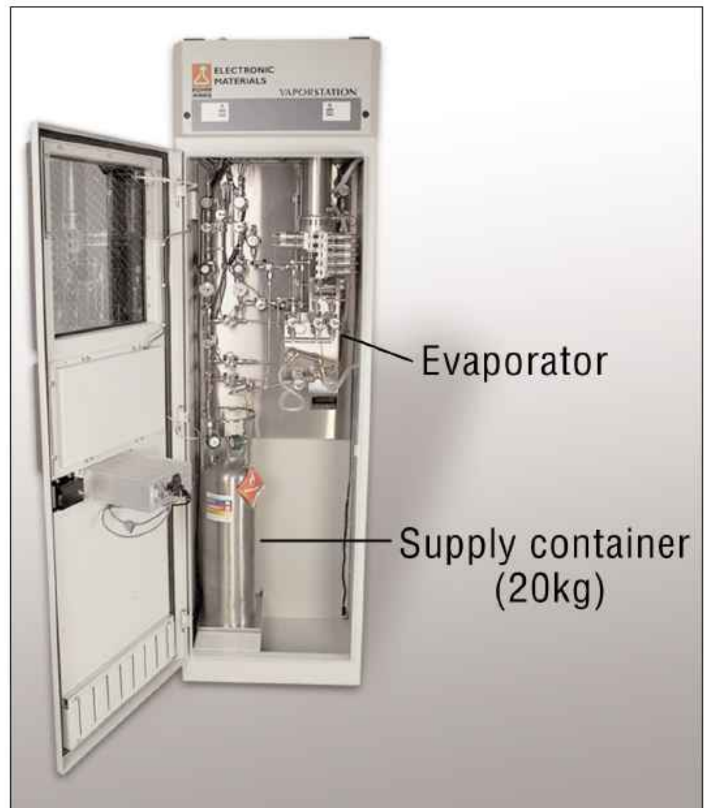
Figure 1. A central vapor delivery system, which uses the same space as a gas cabinet and delivers the vapor of a liquid precursor to several MOCVD reactors.
