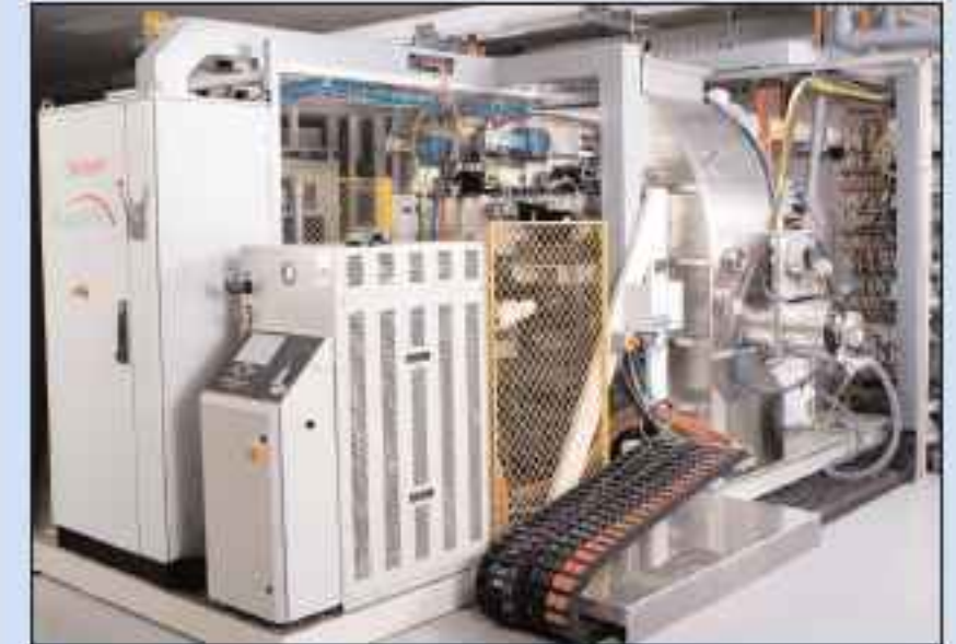
p12 Veeco's new FastFlex web-coating system for manufacturing flexible CIGS PV modules.
