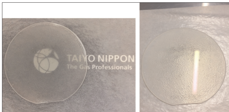
Figure 2. Front side (left): transparent - no unnecessary polycrystals are generated on the wafer edge. Back side (right): since the surface is smooth, the fluorescent light is reflected.
