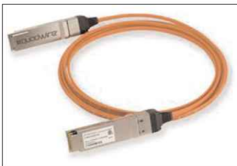
Finisar's 40Gb/s optical link for data centers and computer clusters.
