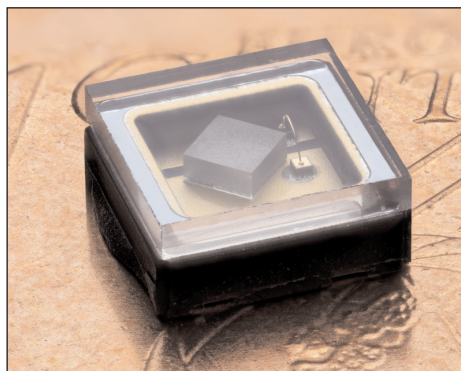
High-power UV-B-LED in package, containing a 1mm x 1mm LED chip.
