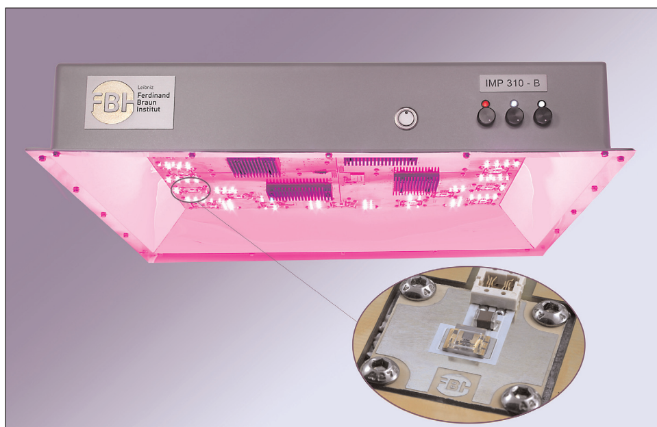
UV-B LED module for plant illumination, providing LED light of three different wavelengths. Brightness and irradiation intensity can be adjusted individually to determine optimum irradiation for structurally diverse vegetable secondary metabolites. Inset: UV-B LED.
