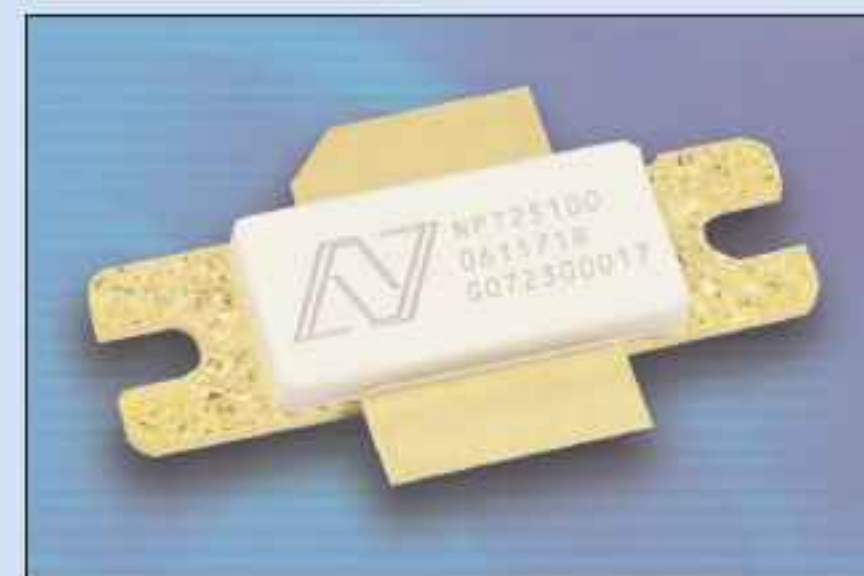
p12 Nitronex's 100 Watt NPT25100 GaN-on-silicon HEMT power transistor for WiMAX applications, launched at the MTT-S event in Hawaii, 3-7 June.
