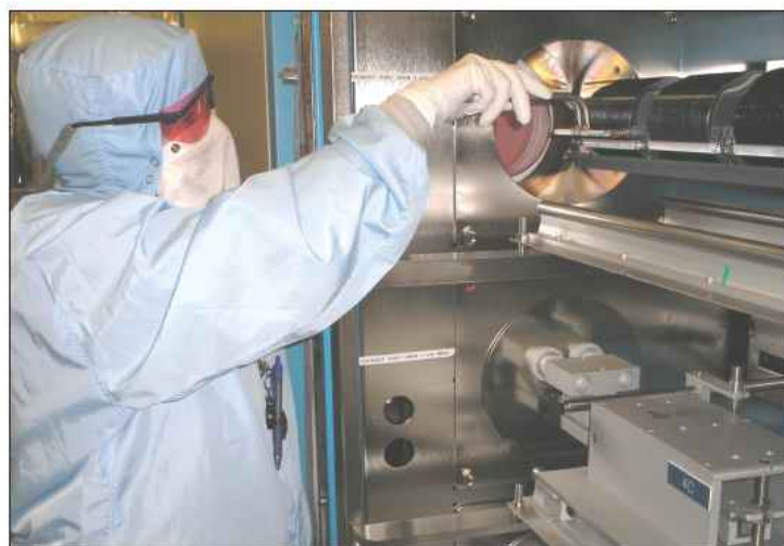
Batches of wafers being loaded into a horizontal furnace in Microsemi's internal fab facility.
