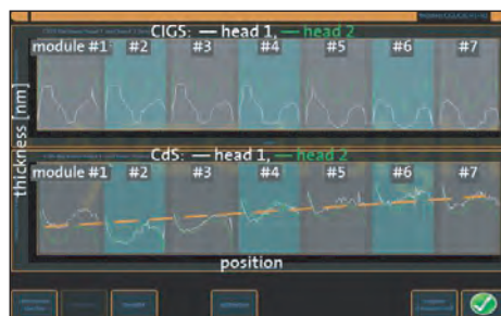
Thickness transients of CIGS and CdS layers by SolR.
