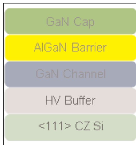
Figure 1: Epi structure of IGaN's GaN-on-Si epi for power applications.
