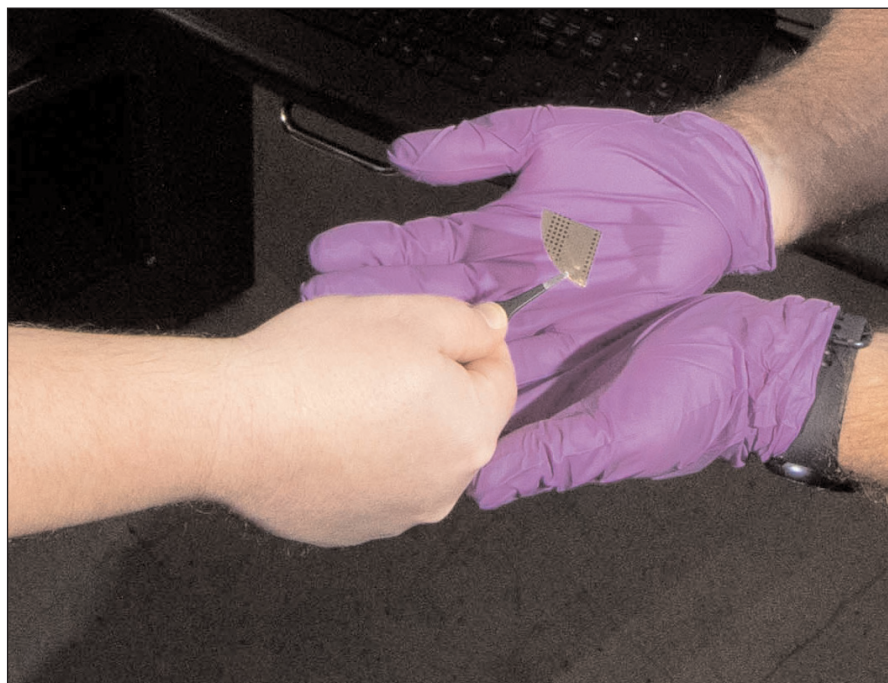
Close-up of Sandia's array of GaN diodes — a step on the path to protecting the electrical grid from EMPs. (Photo by Rebecca Gustaf).
