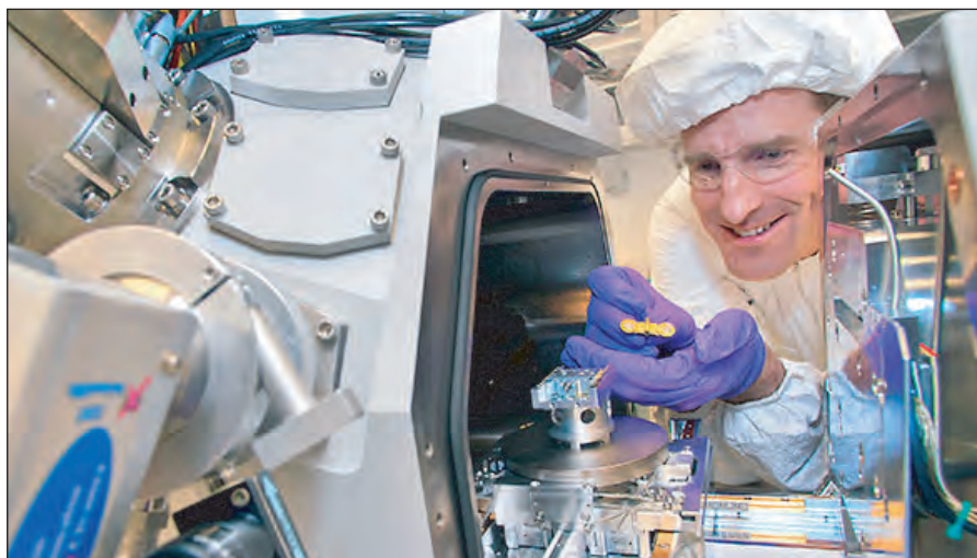
CFN's Kim Kisslinger, here with a focused-ion beam instrument, thinned the InGaN samples to 20nm for electron microscopy.
