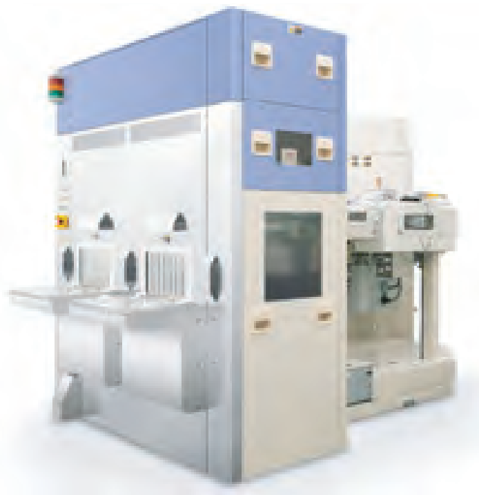
Figure 2. Tokyo Electron's Probus CVD system.
